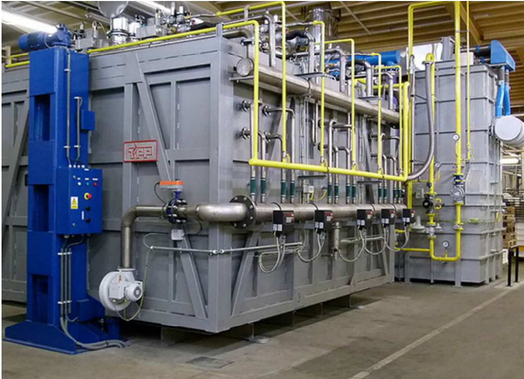
Bell type furnace for firing special ceramics with inert atmosphere 1150 °C
