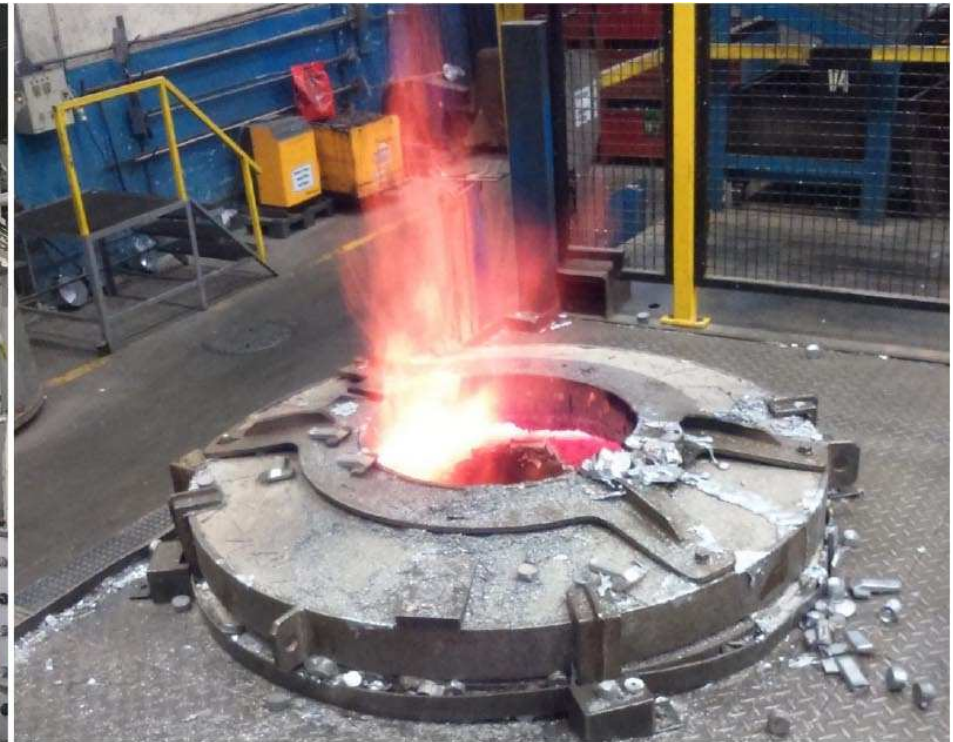
Crucible melting furnace 1 t
