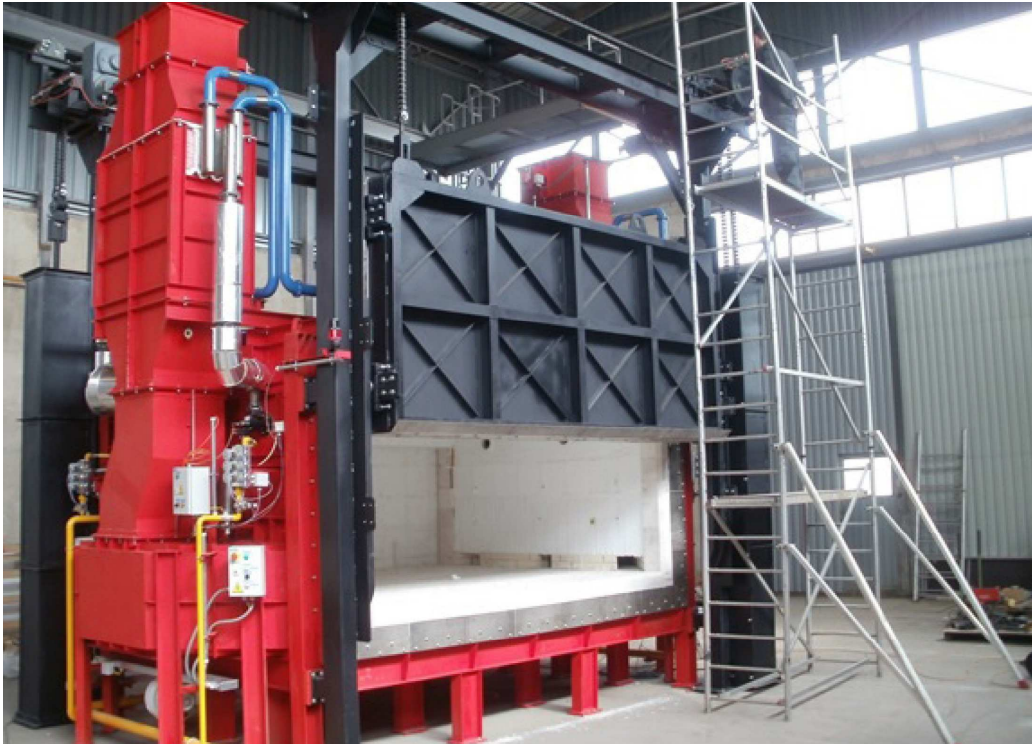
Annealing furnace for titanium products 1150 °C, 7 t, according to AMS 2750E
