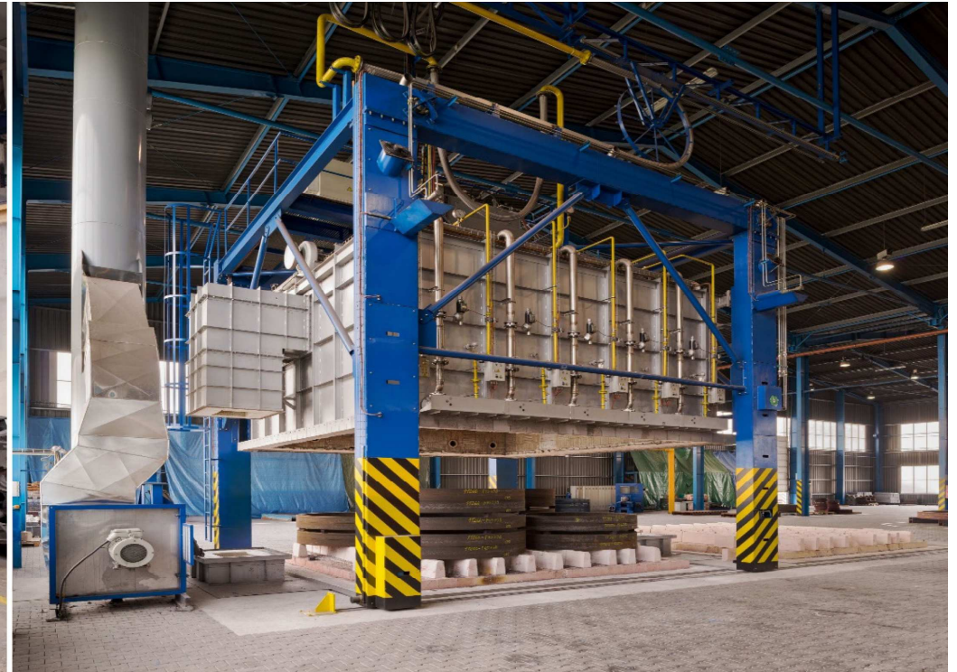
Bell type annealing furnace 1150 °C, 40 t
