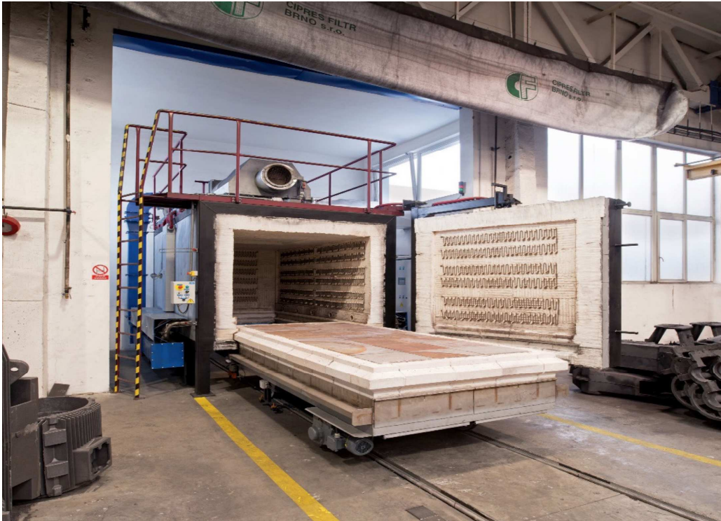
Electric bogie hearth annealing furnace 1150 °C, 5 t
