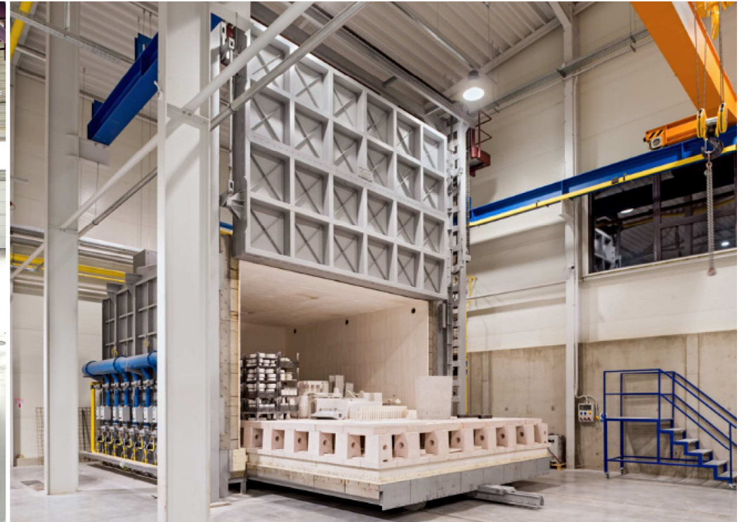
Bogie hearth furnace for firing technical ceramics 1100 °C
