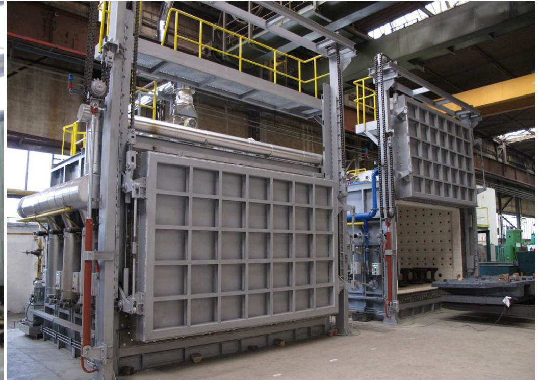
Quenching chamber furnace 1100 °C, 10 t
